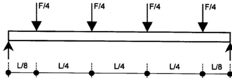
Figure A – Simply supported panel: 4 line loads
